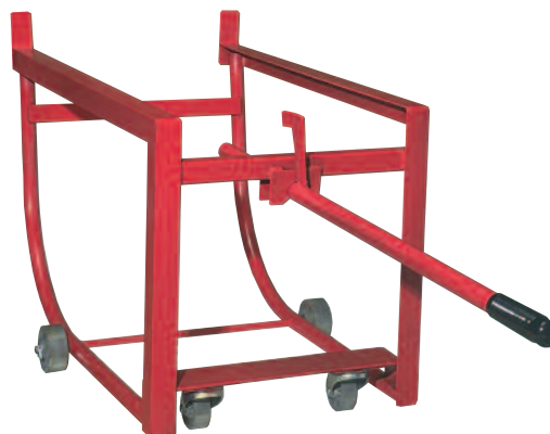
For proper use, simply: 1) lean cradle against drum with nose prongs astride bottom chime; 2) pull out handle and position hook over chime of drum; 3) pull back on handle and drum will seat onto prongs for tipping into horizontal position.
