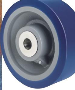
For the extra tough jobs requiring protective polyurethane treads, Hamilton manufactures these top-of-the-line Superlast® Wheels. The extra-thick (1") blue treads (hardness of 90-95 Shore A) are liquid cast and chemically bonded to solid-web, drop forged steel centers. Precision
