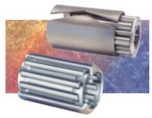
Straight Roller Bearings. Most popular anti-friction bearing for industrial equipment. Consists of a cage-type roller assembly, and an outer race that may be separate or integral. Hamilton most often uses hardened and ground steel roller bearings for maximum loads and life. (Note: plastic retaining washers or other components may be used unless we are advised of a high-heat application.)
