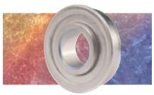
**Ball Bearings.** The standard ball bearings referred to in this catalog are the unground radial type, intended for light-to-medium duty service. On special order we can supply light or heavy-duty precision ball bearings for both radial and thrust loads, In configurations including flanged, sealed, square bores, extended inner raceways, and wide inner raceways with self-locking collars.
