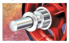
Straight Roller Bearing Seals. A flexible oil-resistant synthetic rubber lip is bonded to the inner circumference of a retaining washer. One such seal-washer is then press-fit into each end of the wheel hub in place of the standard retaining washer. Furnished at no extra cost if specified on Series EHD, CH, A, ES, FM, HS and WH casters; slight extra cost on other caster series or on wheels only. Not available with 11/8" bearings. To order, add suffix -BS to catalog number.
