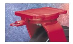
ing control. Springloaded plunger housed beneath caster mounting plate positively engages slots milled in the swivel horn base. When retracted, plunger sits in a vertical notch in the housing to hold it clear of the swivel horn.
