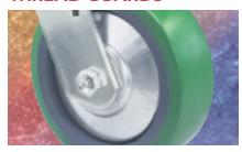
Thread or string guards are fixed discs that fit over the wheel hub to prevent lint, etc. from clogging the axle or bearing. They are always installed in pairs, one on each side of the hub tightened between the spanner bushing and caster legs to prevent rotation. Hamilton offers two series of casters that come standard with thread guards—see pages 46 and 47.
