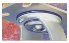
The main and secondary swivel bearing raceways of some Hamilton casters can be ordered with seals by adding the suffix **-SS** to the caster catalog number. Cold-forged Series MS (pg. 28), GS (pg. 29), 52 (pp. 30-31), WW (pg. 32), TG (pg. 46) and TX (pg. 47) can be sealed with special synthetic rubber rings fitted around the circumference of the raceways (illustrated).
