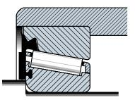
Tapered Roller Bearing Seals are also available with most casters and wheels that offer ¾", 1" or 1¼" tapered bearings. Most often furnished is an integrally sealed assembly supplied by the bearing manufacturer (illustrated), comprising two lips for sealing both O.D. and face (suffix -DS). For certain 1¼" and larger tapered bearings, Hamilton provides a rubber seal and spacer (suffix -CRS).
