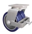
Heavy-Duty Contact Brake.† Newly available on the Maxi-Duty and Dual Wheel Maxi-Duty Casters, this brake is activated by tightening the brake-shoe against the wheel(s). The "thumbscrew" design provides adjustable brake pressure. Add suffix -HCB on Series MD, -DHCB on Series MDD.
