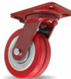
Enhanced Heavy Service (EHS) 600 – 2,000 lbs. Mounting Plate: 4-1/2" x 6-1/2"
