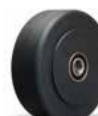
Phenolic (P) & Laminated Phenolic (LP) 1,500 – 4,000 lbs. Standard phenolic wheels up to 16" diameter serve up high capacity at a low cost. Laminated models bolster impact strength by 35% and load capacity by 25%.
