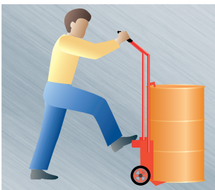
2. Step on foot bar and pull back on handles.
